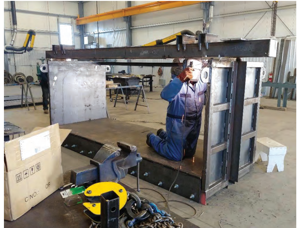
TID's David Bennett secures the hoist mechanism for the Lateral 2 East Horsefly overshoot gate
